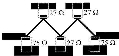
Fig. 9. Microstrip implementation of the filter from Fig. 7.
