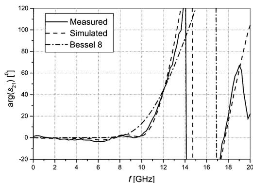
Fig. 11. Residual phase of the transmission coefficient.
