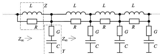
Fig. 6. Half-cell of the complete Gaussian line in an infinite array.
