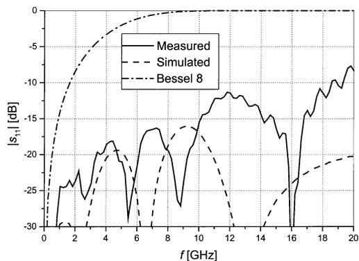
Fig. 12. Magnitude of the reflection coefficient.
