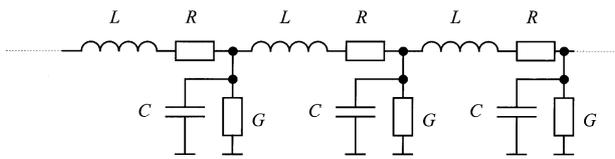
Fig. 1. Lumped-element ladder-network approximation of a lossy transmission line.
