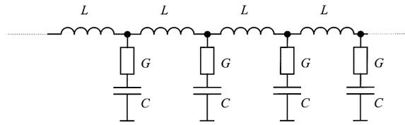
Fig. 3. Lumped-element ladder-network approximation of the incomplete Gaussian transmission line.
