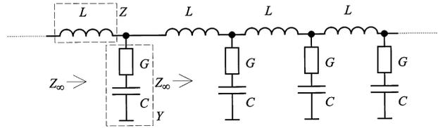
Fig. 8. Half-cell of the incomplete Gaussian line in an infinite array.
